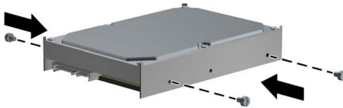
Figure 2-29 Installation des vis de guidage standard
